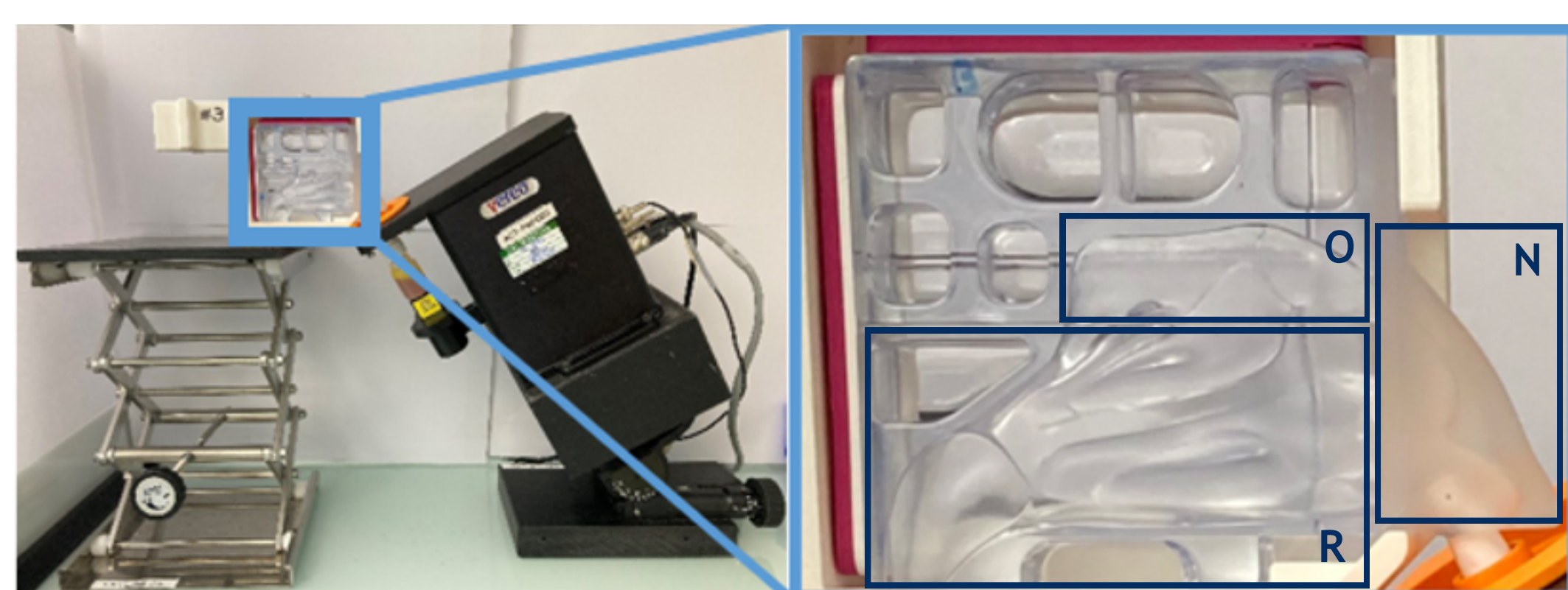
Figure 1 : Deposition testing bench and nasal cast
