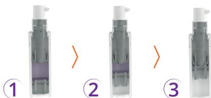
Upon pump actuation, the formulation is dispensed and the bottom piston rises. No air enters in contact with the formulation.
